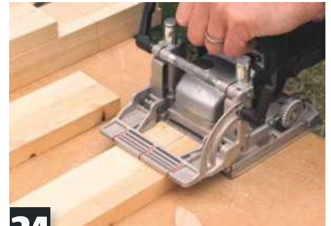
24 Rails and stiles are jointed with No.20 biscuits. Adjust jointer and cut biscuit slots on all timber
